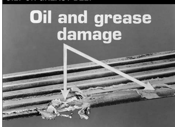
Fig. 13 – Belt ruined by oil and grease soaking
