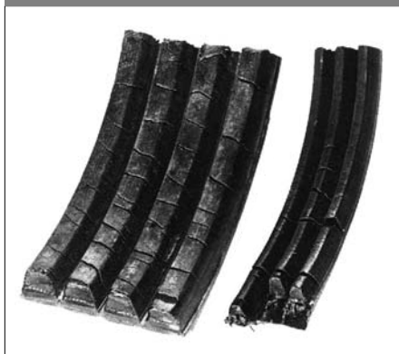
Fig. 20 – Bottom of belts cracking
