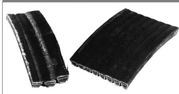
Fig. 21 – Top of band frayed or damaged
