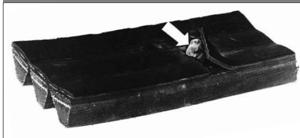
Fig. 23 – Holes or blisters in tie band
